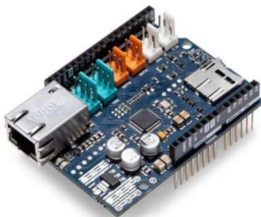
**Figura 5** *Arduino Ethernet Shield 2*
